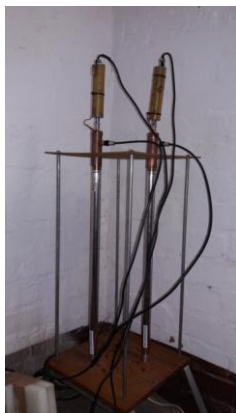
Fig5. Setup used in Freiberg (Germany) in Reiche Zeche shaft Left: Bare counters for the first phase measurements. Right: Counters in borax shield for the second phase measurements.
