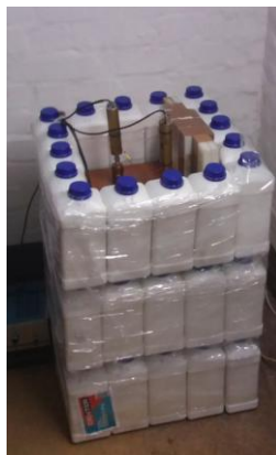
Fig5. Setup used in Freiberg (Germany) in Reiche Zeche shaft Left: Bare counters for the first phase measurements. Right: Counters in borax shield for the second phase measurements.
