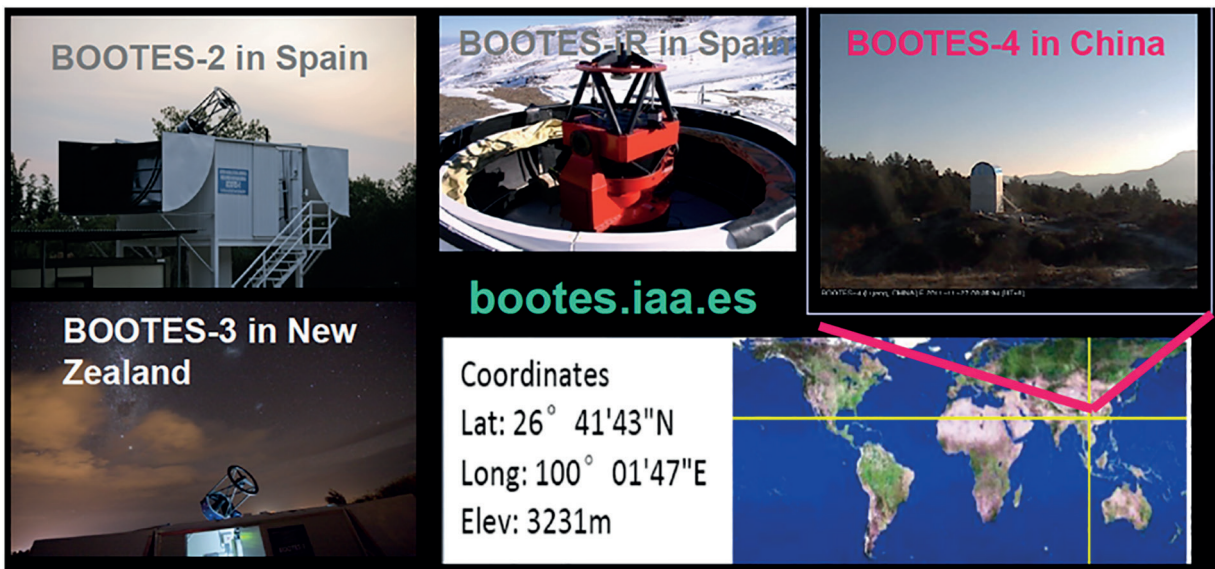
Fig 4. Some of the BOOTES stations worldwide. Robotic telescopes with a diameter of 60cm attached to EMCCD cameras. See [13] for further details.
